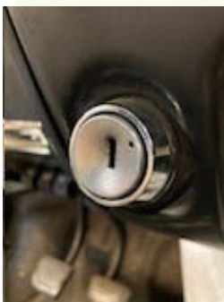
Fig.3 - Image of Internal Vehicle Operation Actuation & Sustainment Lock Cylinder.
