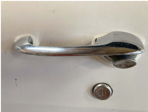
Fig.2 - Image of Human-Powered Piston Actuation Door Release Handle. Note External Key Actuation Lock Cylinder located below Handle casting.
